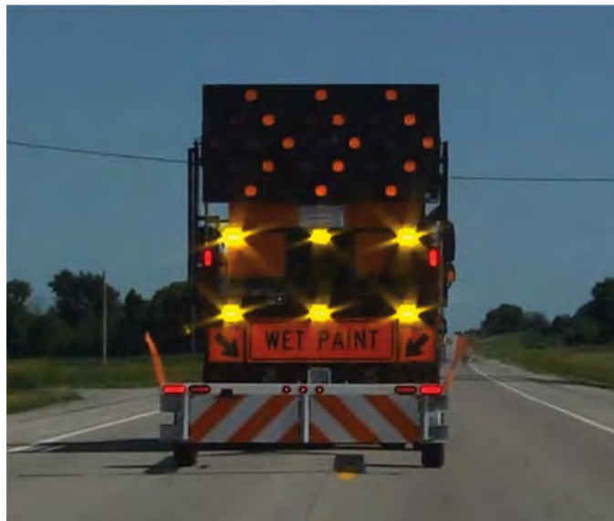
Figure 10. Iowa DOT truck-mounted audible attenuator system (image courtesy of Iowa DOT).
