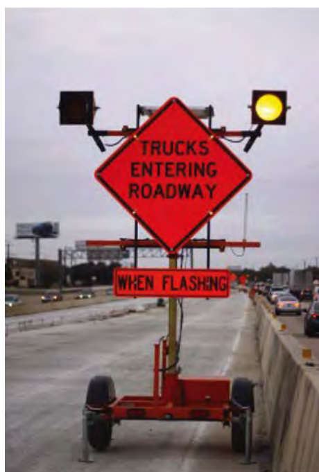
Figure 1. Example of warning sign with LED lights to increase driver attention (image courtesy of SAWS Inc.).
