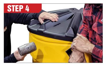
Using the hammer, tap the barrel where the barrel is bulging and preventing the lid from fitting. This should allow the lid to lower onto the snapping point of the barrel.
