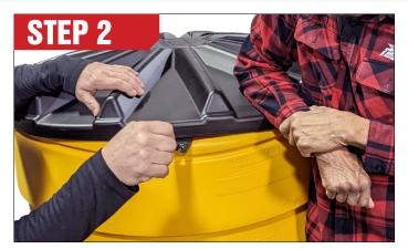
Insert the pry bar between the lid and the barrel. Steadily press down on one side of the lid. Have a second person apply a steady downward force on the lid on the opposite side of the pry bar.
