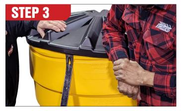
While pressing downward, pull the pry bar downward, flexing the lid outward and pull the lid lower on the barrel. Keep applying the downward pressure.
