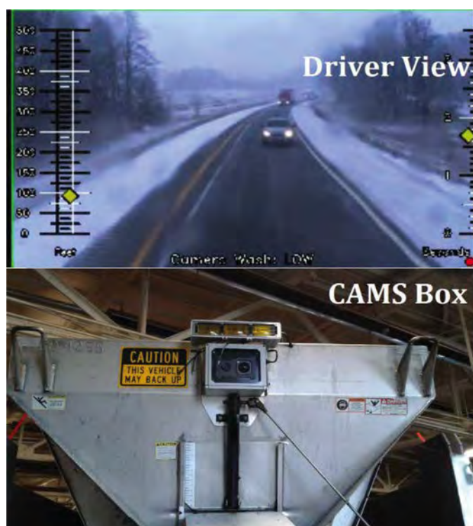
Figure 4. Michigan collision avoidance and mitigation system (Zockaie et al. 2018).
