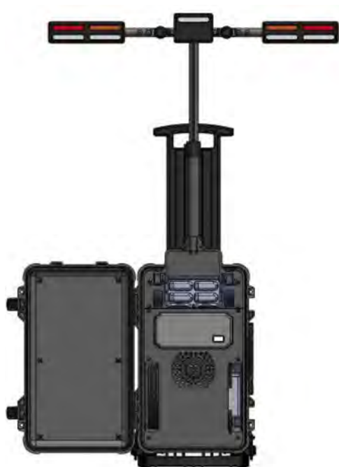
Figure 8. Self-contained intrusion alarm system for flagging operations (images courtesy of Oldcastle Materials).
