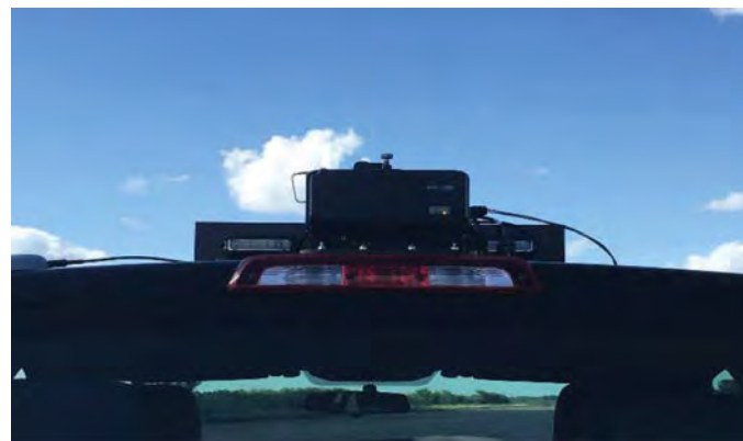
Figure 7. Vehicle-mounted intrusion alarm system for lane closures (Theiss et al. 2017).
