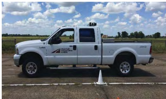
Figure 7. Vehicle-mounted intrusion alarm system for lane closures (Theiss et al. 2017).
