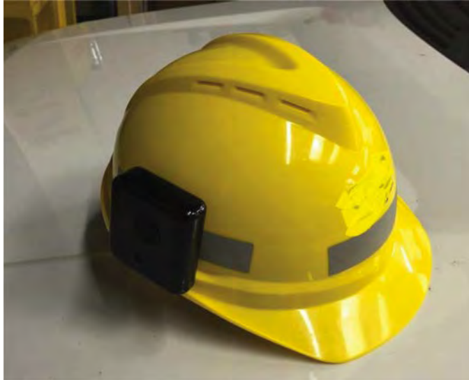
Figure 9. Audible and haptic worker alarm system (Theiss et al. 2017).
