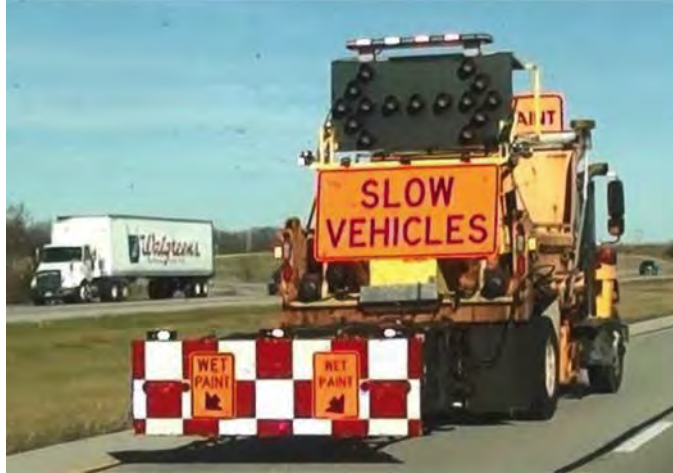
Figure 5. Missouri truck-mounted attenuator with alarm device (Brown et al. 2015b).
