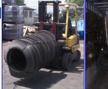
Position lift truck forks approximately 1 foot apart so that forks easily slide through center hole of bundled tires.
